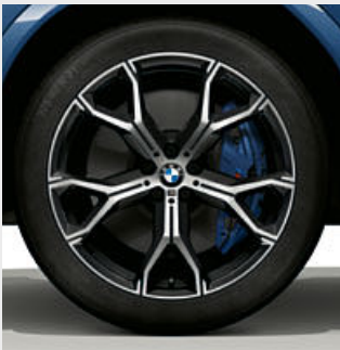
□ 21" M light alloy wheels Y-spoke style 741 M Bicolour Orbit Grey with mixed tyres, gloss-lathed, front 9.5J x 21 with 275/40 R21 tyres, rear 10.5J x 21 with 315/35 R21 tyres. 2, 3, 6
