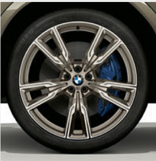
□ 22" M light alloy wheels V-spoke style 747 M Cerium Grey matt with mixed tyres, gloss-lathed, front 9.5J x 22 with 275/35 R22 tyres, rear 10.5J x 22 with 315/30 R22 tyres. 5, 6
