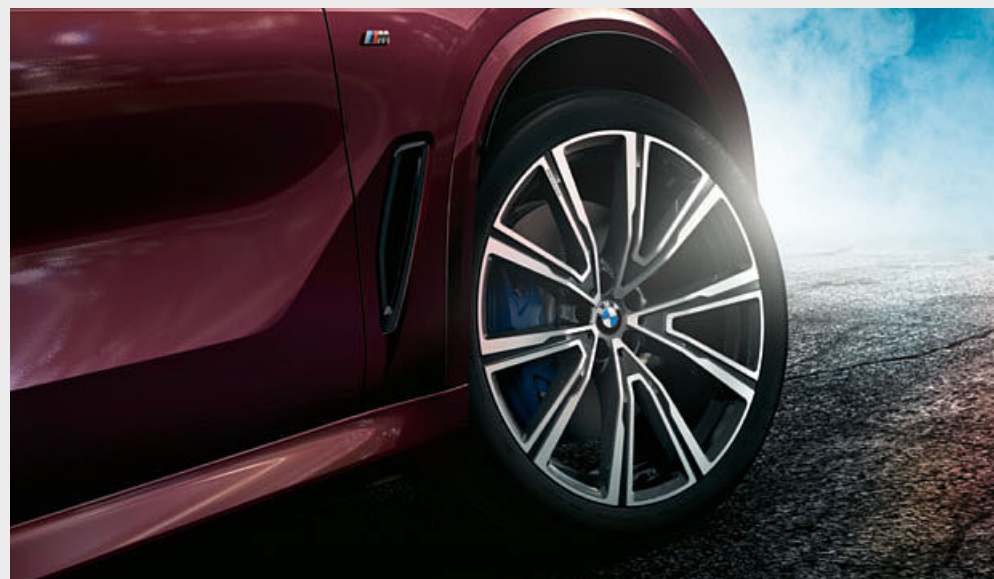
□ 22" BMW Individual light alloy wheels V-spoke style 746 I Orbit Grey with mixed tyres, front 9.5J x 22 with 275/35 R22 tyres, rear 10.5J x 22 with 315/30 R22 tyres.
