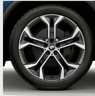
□ 21" light alloy wheels Y-spoke style 744 Bicolour Orbit Grey with mixed tyres and runflat tyres, front 9.5J x 21 with 275/40 R21 tyres, rear 10.5J x 21 with 315/35 R21 tyres. 1,5
