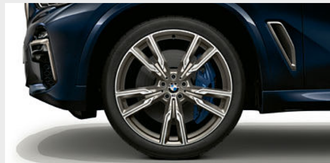
□ 22" M light alloy wheels V-spoke style 747 M Cerium Grey matt with mixed tyres, front 9.5J x 22 with 275/35 R22 tyres, rear 10.5J x 22 with 315/30 R22 tyres. 3,5
